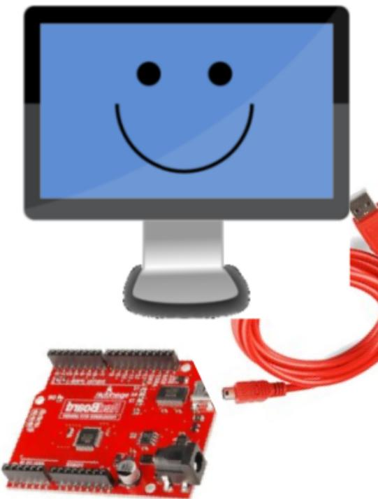
Data passes between the computer and Arduino through the USB cable. Data is transmitted as zeros ('0') and ones ('1') sequentially.
